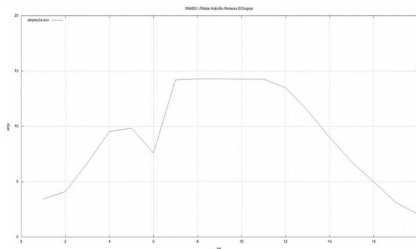
Figure 4 – An overdense meteor profile generated by “Rambo”.
